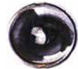
Traditional O-Ring Traditional O-Ring after 50,000 test cycles is non-functional.
